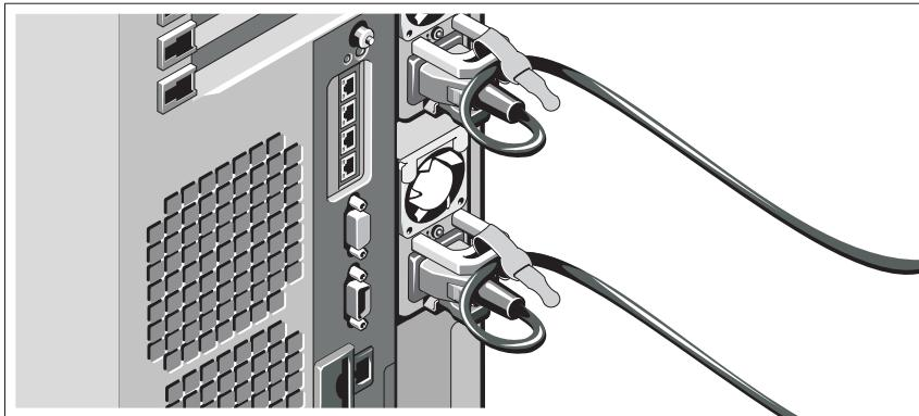
Bend the system power cable(s) into a loop as shown in the illustration and secure the cable with the provided strap.
